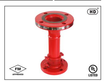
The inlet of foam maker is designed to create venturi jet which draws air into the foam solution stream. The air is drawn into the foam solution through holes located on the foam maker covered with stainless steel screen to exclude nesting birds and insects. The aerated foam is directed into the pourer for the gentle application of the expanded foam. The pourers are available in different models.\*
